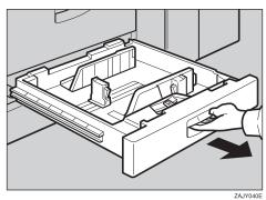
While pushing the release lever, adjust the side fences and back fence to the new paper size.
